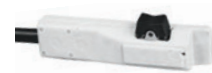
RMLS-14 Switch 129337 Momentary- and maintained-contact rocker switch for contactor control. Push forward for maintained contact and backward for momentary contact. Includes 26.5-foot (8 m) cord and 14-pin plug.
